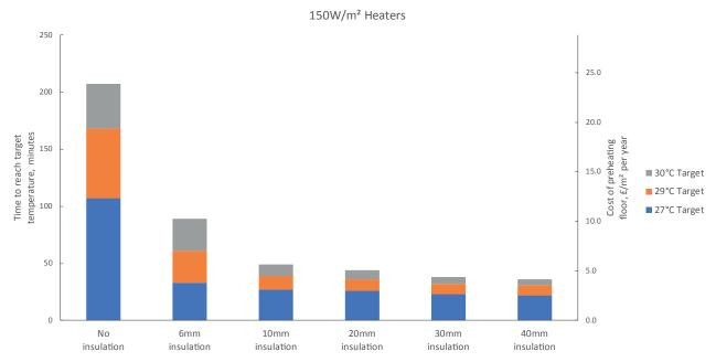
Using Warmup insulation boards decreases heat up time by at least two times (comparing no insulation vs 6mm insulation) It can take as little as 35 minutes to reach 30°C floor temperature with Warmup insulation boards! For comparison for a floor without insulation to reach 30°C, it could take up to 3 hours and 20 minutes! That's 2 hours and 45 minutes of wasted energy. (Comparison made between 40mm insulation and no insulation).
